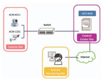
With remote monitoring can review the information from the cameras in real time without exhausting the resources of the network. It is like the supervisor can be in two places at one time. Another advantage of using ACTi cameras system is to downrate the theft, the IP cameras can provide valuable evidence to identify the thief in high quality image. Besides, the ACTi NVR allows recording simultaneous images of the cameras or selecting the required image in HD quality.
