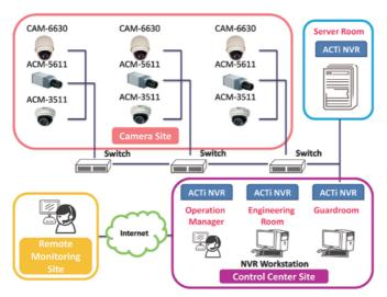
transmitted via internet network. Thanks to the PoE support of ACTi cameras, power delivery and the data transmission are completed over one single network cable and therefore decrease the overall installation expenditures. All the cameras are linked to "Linksys Full POE Gigabit Switches". In the core of system, CISCO Full Fiber 3750 Series Switch is used. The whole complex is put in action and allows Security Office to monitor all the IP cameras installed throughout the production area.
