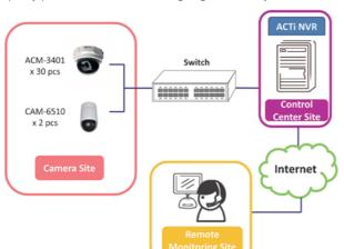
CAM-6510 completed the whole surveillance system. It patrols the whole casino and even any emergency occurs, the camera can instantly zoom in optically. The ACTI NVR Enterprise allows to have live-view as well as to retrieve recorded videos remotely and conveniently. Using the Internet Explorer browser, all cameras can be live-viewed on the two flat screen monitors installed at the rest and smoking zone.
