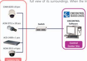
their surveillance system, some traditional analog cameras were converted to IP by using the ACD-2400 video encoder. Indar chose CIRCONTROL software along with ACTI IP cameras to have the best image quality for recognizing the car plate in order to control the vehicular traffic.
