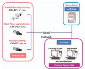
parcels way from incoming gate to delivery car. If parcel is lost, the administrative staff can always check when and how the mistake was made and how to improve service quality. To monitor large parts of technology line, ACM-5601 Megapixel box camera is used; for fast moving parts, ACM-5711 is used.
