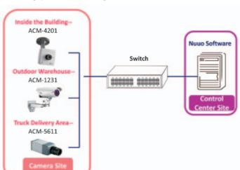
Besides, the all-in-one outdoor camera ACM-1231 is equipped with IR LED provides the best quality of images even in the night time. These cameras are PoE supported which the data and the power supply can be transmitted via single network cable. However, the most important reason that ACTi was chosen is that ACTi offered the best price/ performance solution to the end user
