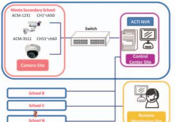
system is managed by ACTi NVR software. All the FTS schools' surveillance system will be connected by ACTi CMS software from the control center.
