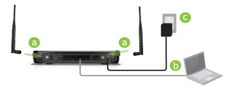
a) Attach the antennas of the High Power Repeater to the antenna ports labeled 1 and 2
