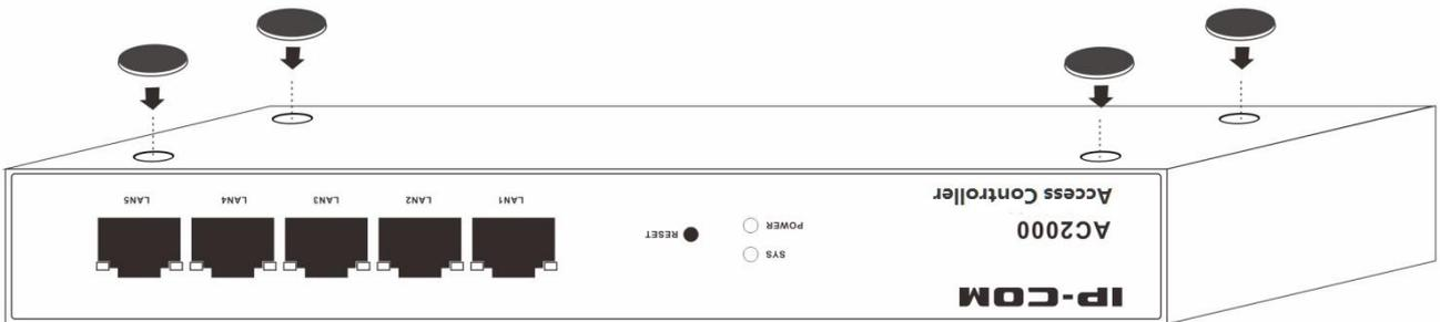
Step 3: Flip the access controller for placement on the workbench with face up.
