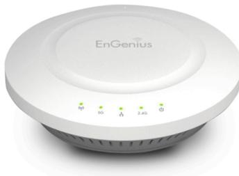
**EAP600** is a wireless-11n 600Mbps (300Mbps + 300Mbps) High Power Dual Band concurrent ceiling mount AP. It allows simultaneous operation of 2.4GHz and 5GHz wireless network. With media-optimized performance, you can enjoy internet surfing more smoothly and with less lag.
