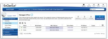
B) You may configure your Managed AP(s) after you successfully connected to the Wireless Management Switch through its GUI.
