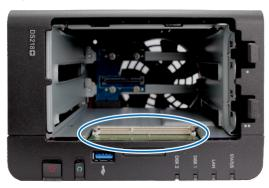
*Important:* When you remove the drive trays, you expose sensitive internal components. Avoid touching anything other than the memory assembly when you remove or add a memory module.
