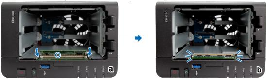
Important: Hold the memory module by its edge, and do not touch the gold contacts.
