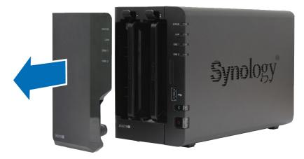
2 Push the latch upward and pull the handle to remove the drive tray from your DiskStation.
