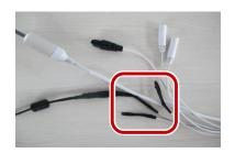
Connect the tail cables, and protect the cables and cable connections using insulating tapes. Then wrap all the tail cables together using insulating tapes.
