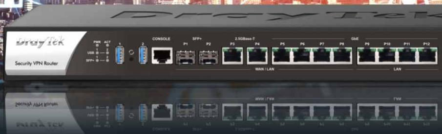
Vigor3912 is designed for bandwidth-demanding networks, featuring a 2GHz Quad-Core CPU for fast connection speed, even with multiple connected devices. The router has 8 WAN interface, including 2x 10G SFP+ for fiber connectivity, 2x 2.5G Ethernet, and 4x 1G Ethernet. Port1 to port8 are configurable independently for WAN or LAN to offer flexibility and optimize the router performance.
