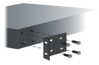
2. Then, install the Vigor router (with rack mount kit) on the 19-inch chassis by using other four screws.
