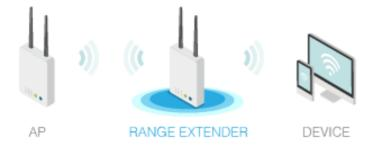
The access point can act as a wireless repeater; it can be Station and AP at the same time. It can use Station function to connect to a root AP and use AP function to serve all wireless stations within its coverage.
