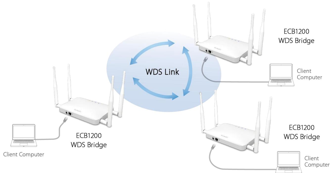
**Note:** WDS Bridge Mode does not act as an Access Point. Access Points linked by WDS are using the same frequency channel. More Access Points connected together may lower throughput. This configuration can be susceptible to generate endless network loops in your network, so it is recommended to enable the Spanning Tree setting (see 6.3 Spanning Tree Setting, below) to prevent this from happening.
