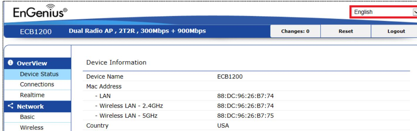
The screenshot shows the EnGenius web interface for the ECB1200 device. The language dropdown menu is highlighted with a red box and shows "English" selected. The main content area displays "Device Information" with the following details:
