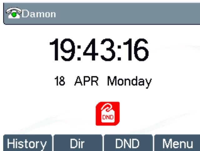
**Figure 46 - DND Enabled on All Lines**
