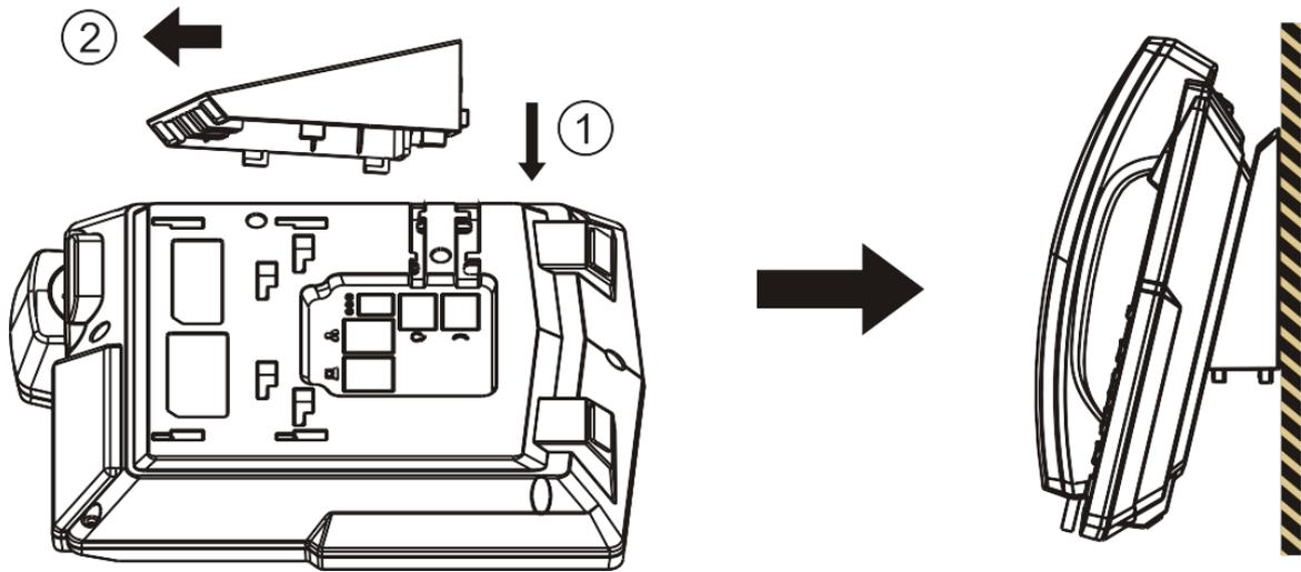
**Figure 2 - Wall-mount Installation**
