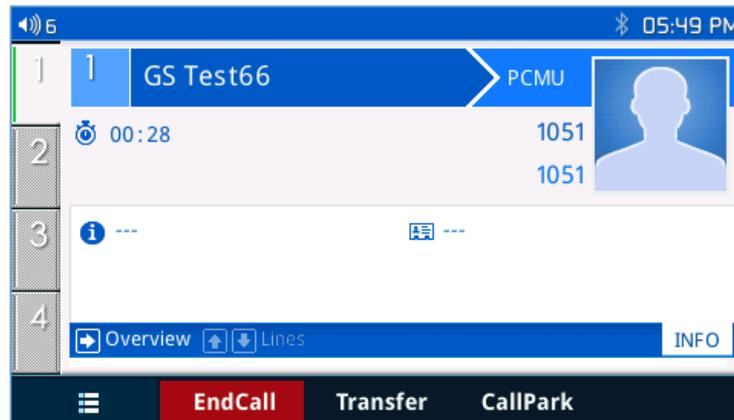
Figure 3: Transfer Softkey During Call
