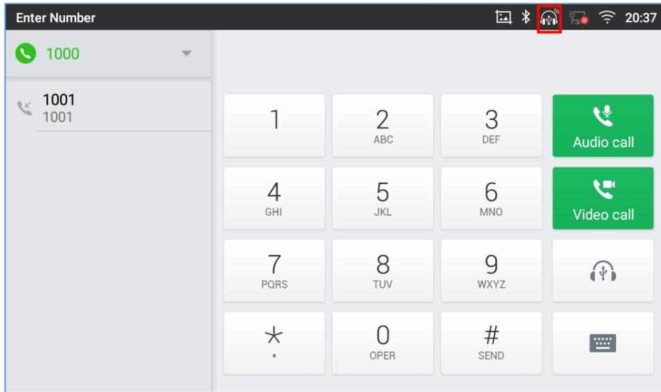
**Figure 128: USB Headset Used for Call**
