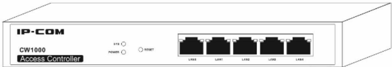
**Step 2:** Connect the LAN port of the AC to the remote Ethernet device, such as a switch, router, AP, etc.
