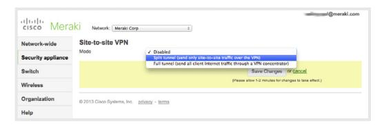
Split tunnel mode will only send site-to-site traffic over the VPN, leaving other traffic (such as direct Internet requests) to be directed to its final destination without needing to go through the secure VPN tunnel. In other words, email or file server requests between two offices would traverse the split tunnel VPN; a user's request to view a website such as www.nytimes.com would not.
