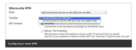
If configuring a mesh topology, ensure every participating MX has the "Connect directly to all peers" option selected. If configuring a hub-and-spoke topology, ensure that the hub MX is configured to mesh to all peers, while every branch ("spoke") MX is configured to "Connect directly to only one VPN peer (hub-and-spoke mode)":
