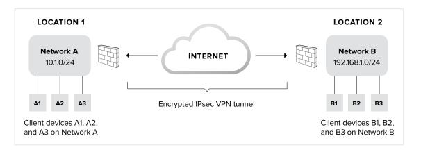
Site-to-site VPNs are deployed between the security appliances/firewalls at each location. The client devices (such as laptops or workstations) behind these firewalls do not need software installed or local settings configured to enable them to send or receive data with the other sites.
