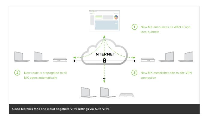
That Auto VPN leverages the cloud in this unique, intelligent way means less manual configuration and time spent by IT admins to set up VPN tunnels between sites, and fewer opportunities to introduce human error into the process.
