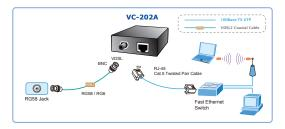
Figure 3-6: Connecting Multiple PCs to an Ethernet LAN
