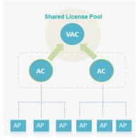
Figure 11: Virtual AC Enabling Centralized Management
