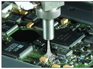
Figure 6: Conformal Coating Protection
