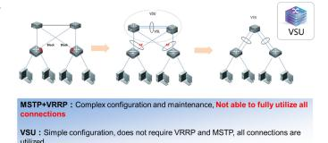
Figure 4: Simplified Network Topology Enabled by VSU
