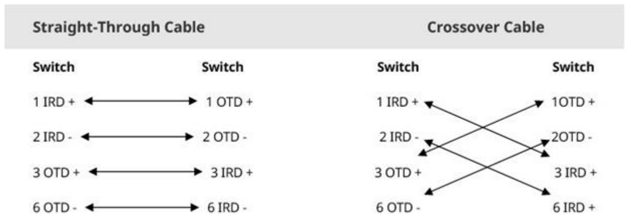
Figure 7-3 100BASE-TX/10BASE-T Twisted Pair Connections
