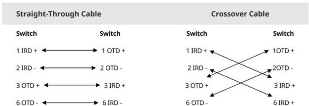
Figure 7-3 100BASE-TX/10BASE-T Twisted Pairs Connection
