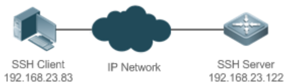
Figure 1-1 Networking Topology of SSH Device Management
