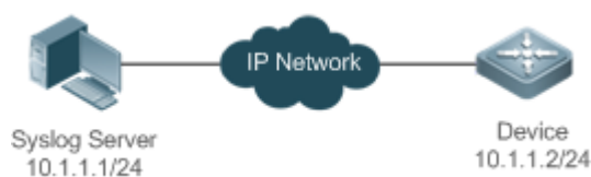
Figure 1-2 Networking Topology of Sending Syslogs to the Log Server
