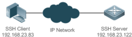
Figure 1-5 Networking Topology of SSH File Transfer
