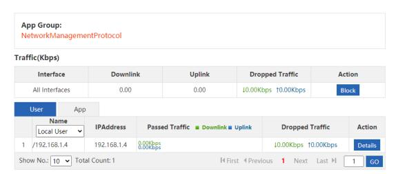
This window displays the application group and type of the selected application, the uplink/downlink traffic occupied by the selected interface, the traffic dropped by the rate limiting policy, and the traffic of the user that runs this application.
