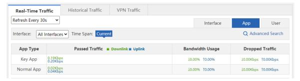
Traffic analysis of key/guaranteed applications: Display the details of key/guaranteed applications on the selected interface, the traffic usage of each application, details of users running the key/guaranteed applications, and the traffic usage of each user.
