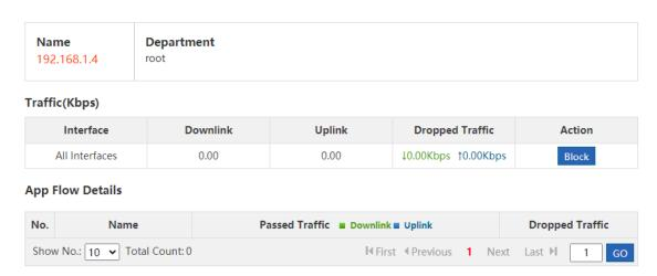
You can click to block the traffic of the current user. After blocking, the subsequent traffic of this user is completely dropped by the selected interface.
