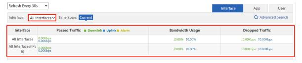
According to the traffic information displayed in the figure above, you can check whether the current traffic is normal (whether any alarm occurs). If the traffic is too high, a yellow alarm — Alarm occurs, which helps you quickly locate the bandwidth problem.
