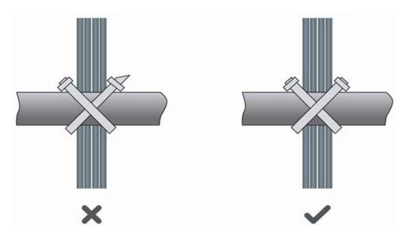
• When cables need to bend, you should first bundle them up. However, the buckle cannot be bundled within the bend area. Otherwise, significant stress may be generated in cables, breaking cable cores. As shown in Figure D-3.
