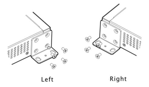
Use the expansion screws to secure the mounting brackets on the wall, as shown in Figure 3-5.
