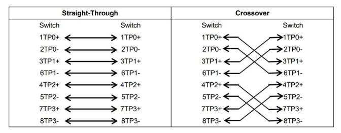
In addition to the above cables, the 100BASE-TX/10BASE-T can also use 100-ohm Category-3, 4, 5 cables for 10 Mbps, and 100-ohm Category-5 cables for 100 Mbps, both of which can be up to 100 m. Figure A-2 shows the pinouts of the 100BASE-TX/10BASE-T.
