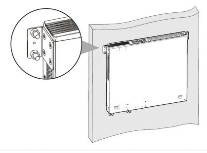
A SUITABLE FOR MOUNTING ON CONCRETE OR OTHER NON-COMBUSTIBLE SURFACE ONLY.
