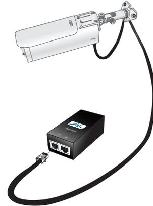
2. Connect an Ethernet cable from your LAN to the Ethernet port labeled **LAN** on the *PoE Adapter*.
