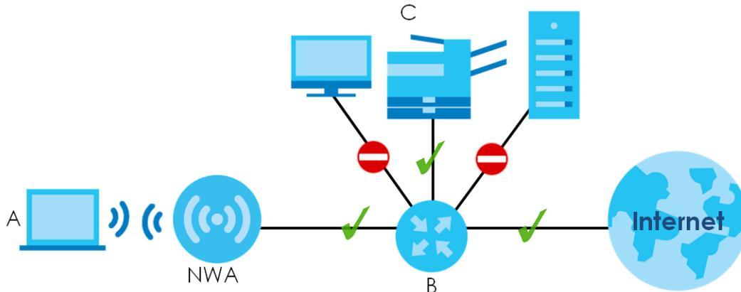
MAC addresses that are not listed in the layer-2 isolation table are blocked from communicating with the Zyxel Device's wireless clients except for broadcast packets. Layer-2 isolation does not check the traffic between wireless clients that are associated with the same AP. Intra-BSS traffic allows wireless clients associated with the same AP to communicate with each other.
