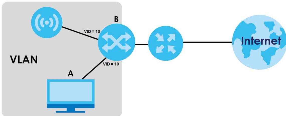
In the figure above, to access and manage the Zyxel Device from computer **A**, the Zyxel Device and switch **B**'s ports to which computer **A** and the Zyxel Device are connected should be in the same VLAN.
