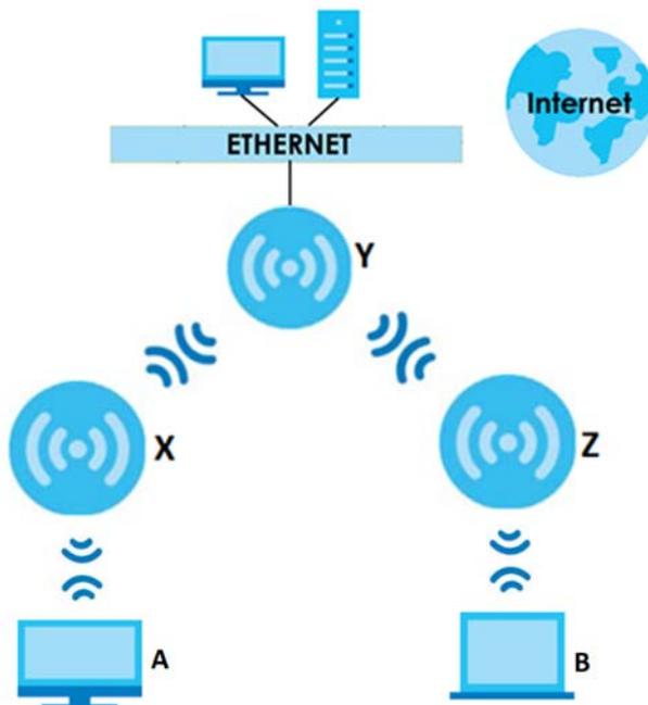
The following figure shows an example of a wireless bridge network. The root AP (Y) is connected to a network with Internet access and has a wireless repeater (X) connected to it to expand the wireless network's range. Clients (A and B) are connected to the wired network through the gateway (G). They can access the wired network through the wireless repeater and/or root AP.
