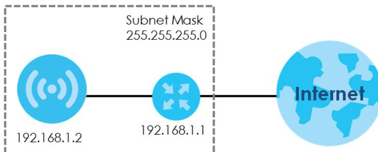
The figure above illustrates one possible setup of your Zyxel Device. The gateway IP address is 192.168.1.1 and the managed IP address of the Zyxel Device is 192.168.1.2 (default), but if the Zyxel Device is assigned an IP address by a DHCP server, the default (192.168.1.2) will not be used. The gateway and the Zyxel Device must belong in the same IP subnet to be able to communicate with each other.
