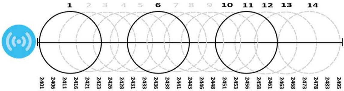
Three channels are situated in such a way as to create almost no interference with one another if used exclusively: 1, 6 and 11. When an AP broadcasts on any of these 3 channels, it should not interfere with neighboring APs as long as they are also limited to same trio.
